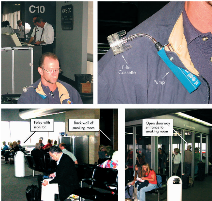
Figure 2 Lambert-St Louis International Airport nicotine monitor test, conducted Thursday, 26 September 2002. Pump assisted nicotine monitor test conducted roughly 35 feet (10 m) from front wall containing the entrance to smoking lounge 4C. The test ran for four hours from 1.30 pm to 5.30 pm. The first three photos show James Foley of Environmental Solutions conducting the test in the seating area adjoining gate C10 on the C Concourse. The fourth photo shows the smoking room, the entrance to which faces the corridor leading down the concourse.
