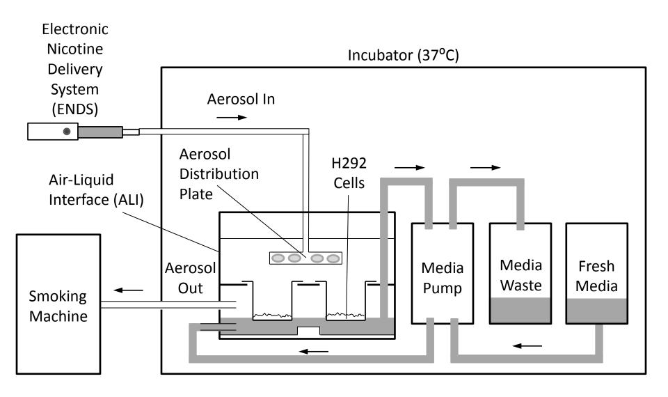
**Supplemental Figure 1.** Air-liquid interface (ALI) exposure system of bronchial epithelial cells to ENDS aerosol. **Note**: Items are not to scale.
