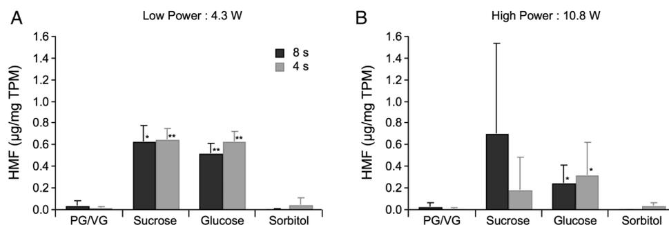
**Figure 1** Average HMF yield normalised by TPM (µg/mg) in aerosols generated from laboratory-prepared sucrose, glucose and sorbitol liquids vaped at 4.3 W (A) and 10.8 W (B) and at 8 and 4 s. \* and \*\* indicate significant difference from the unflavoured liquid at  $p < 0.05$  and  $p < 0.01$ , respectively.  $N = 3$  measurements for each condition. FA, furfural; HMF, 5-hydroxymethylfurfural; PG, propylene glycol; TPM, total particulate matter; VG, glycerin.
