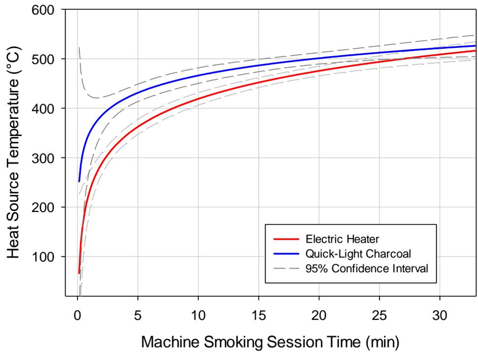
**Figure S-2. Heat source temperature curves fitted to averaged thermocouple data collected during machine smoking of the Research-Grade Waterpipe using electric and charcoal heating.**
