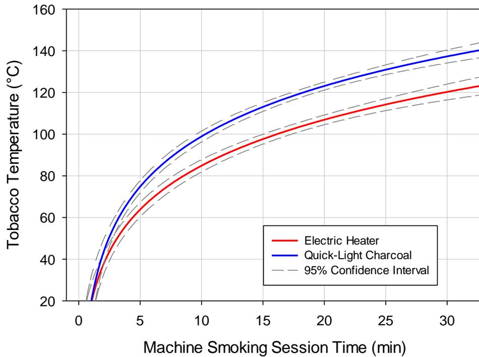
**Figure S-1. Tobacco temperature curves fitted to averaged thermocouple data collected during machine smoking of the Research-Grade Waterpipe using electric and charcoal heating.**
